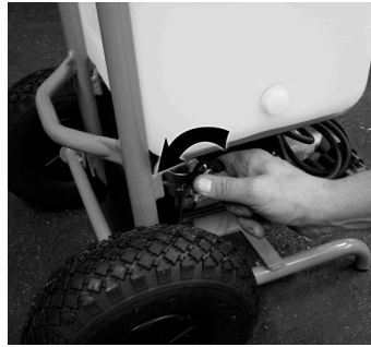
2. Fill tank and open ball valve
