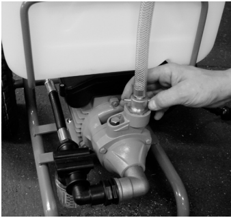
1. Connect pressure hose to pump outlet
