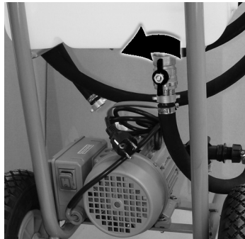
4. Fill container and open the ball valve.
